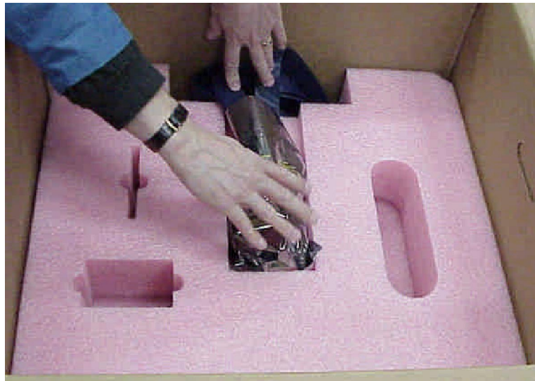
Figure 1-14: Place the probe head into the square cutout
